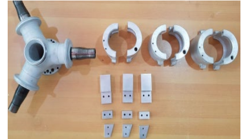
Civil and Airforce Airplane; Cadmium & Hard Chrome Truboprop Parts and Blade Aluminum Anodizing
